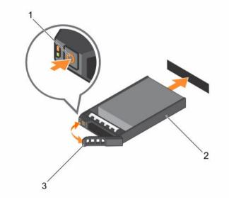
Figure 24. Removing and installing a hot-swappable hard drive/SSD
